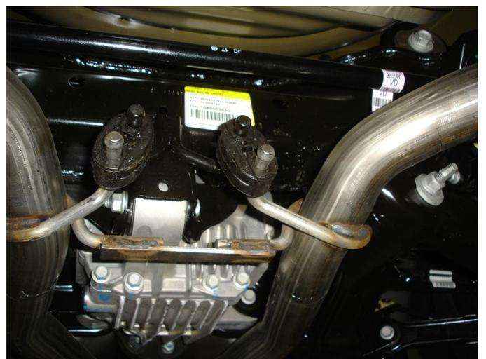
**Step 2.** To remove the OEM exhaust loosen the two bolt clamps located behind the catalytic converters. Working rearward disengage the rubber insulators from the welded hangers, retain clamps and rubber insulators as they will be used to install the new system. Remove complete system.
