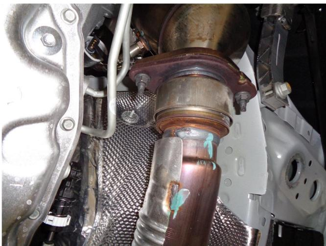
**Step 1.** To remove the OEM exhaust you will need to unbolt and remove the cross brace shown. Now you can unbolt the OEM exhaust from the catalytic converter flange junction. Disengage all welded hangers from the rubber insulators. Retain rubber insulators as they will be needed to install your new MAGNAFLOW system. The OEM system can now be removed.
