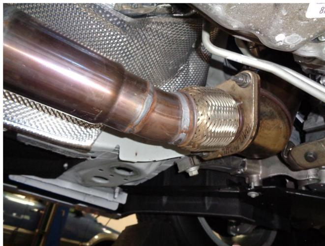
**Step 2.** Begin installation of your new MAGNAFLOW system by loosely bolting the Inlet Pipe Assembly to the catalytic converter outlet flange using the OE fasteners.
