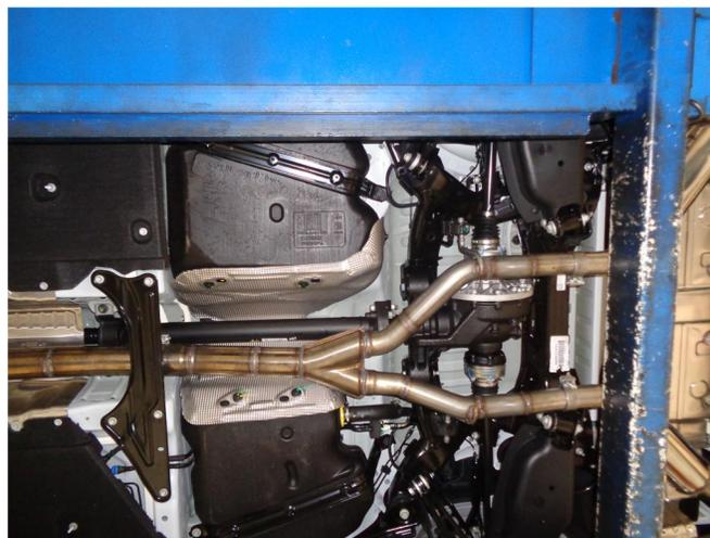
**Step 3.** Next, loosely install the Y-Pipe Assembly using the supplied 3.00" clamps. Locate the welded hangers to the rubber insulators.
