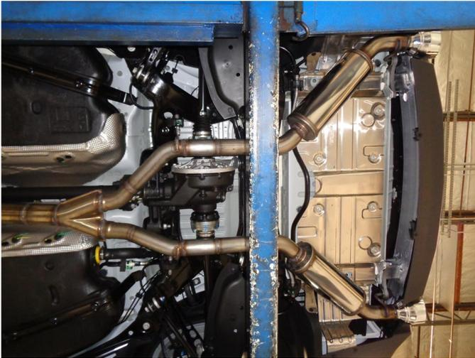
**Step 4.** Loosely install the drivers and passengers side Muffer Assemblies using the supplied 2.25" clamps. Engage the welded hangers to the rubber insulators.
