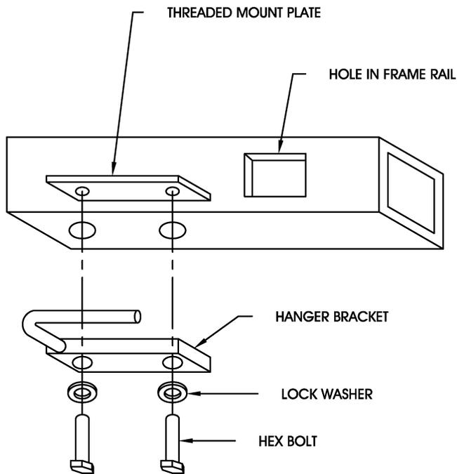
**Step 4:** Once a final position has been chosen for the new system, evenly tighten all fasteners from front to rear. The supplied band clamps must be VERY tight to properly align the pipes and prevent leaks (Approximately 40ft-lbs). U-bolt clamps should be tightened to approximately 30-35ft-lbs. Inspect all fasteners after 25-50 miles of operation and retighten if necessary.
