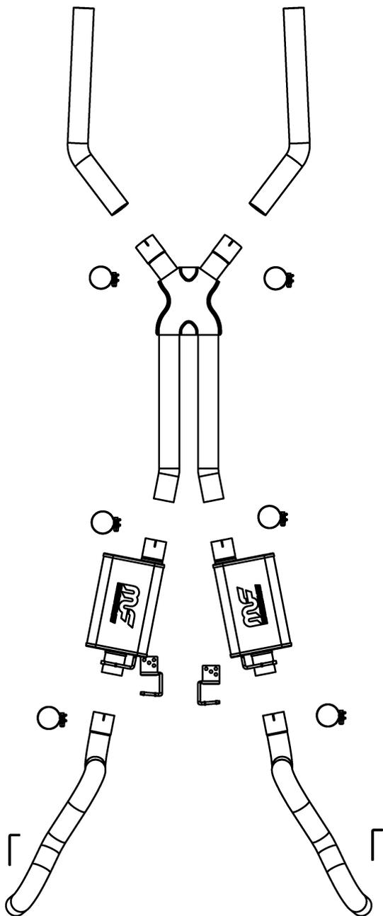
*Note: This system is designed to work with OEM-style exhaust manifolds, or tubular headers. Due to the various applications possible, some modification and welding is required for a proper fit and finish.*
