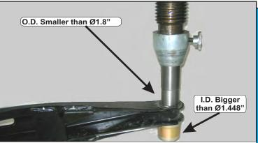
I.D. of rear lower control arm inner position is Ø1.448". Using a hydraulic press, properly support control arm and slowly push out the rubber bushing with bonded outer metal shell. Remove all sharp edges from I.D. Apply grease to all metal parts that will contact the new polyurethane bushings.
