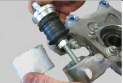
Refer to the shop manual for the safe removal of front and rear control arms, torque specs, and alignment of your vehicle. Removal of the factory bushings on the trailing arm, adjuster link & knuckle will all be the same. The bushings are not bonded & no metal shell to press out.
