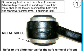
Refer to the shop manual for the safe removal of front and rear control arms, torque specs, and alignment of your vehicle.
