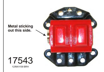
Assemble the two half together with the supplied nuts, bolts and washers. Install the bolts from the bottom with the washers and nuts on top. HINT: Due to the many different metal configurations from foreign and domestic manufacturers it maybe helpful to apply a thin coating of grease or dishwashing detergent to the polyurethane insert, at metal contact points before installing. This will allow the insert to seat, in turn allowing proper bolt alignment.
