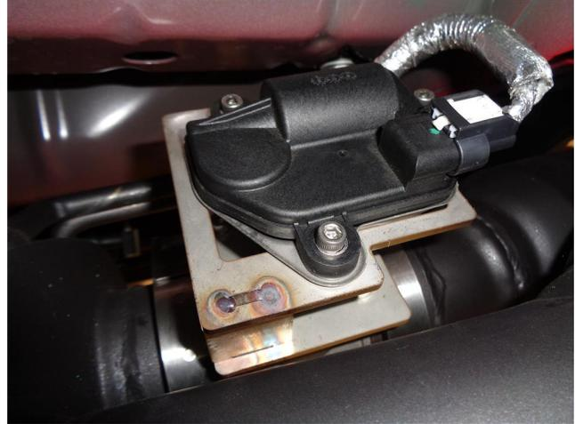
**Step 4.** Valve orientation should be placed with the electrical plug facing the rear of the vehicle. Rotate valve to be free of any interference like the body, exhaust system or hangers that can damage the valve. Once a final position has been chosen for the new valve system, evenly tighten all clamps from front to rear. Re-connect the wiring harness plug to the Valve motors and wire mounting bracket. Inspect all fasteners after 25-50 miles of operation and re-tighten if necessary.
