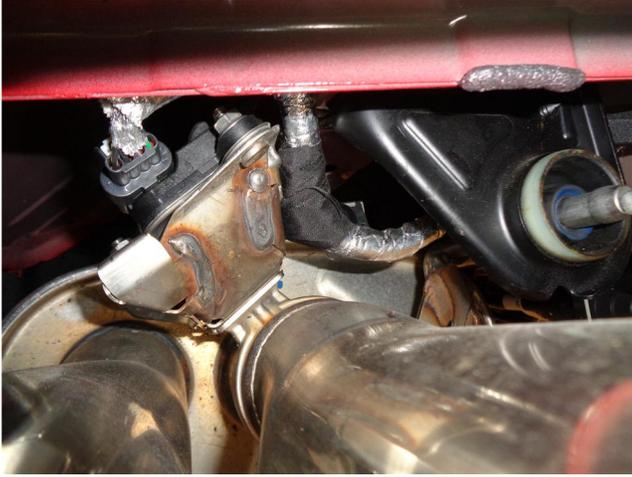
**Step 1.** Unplug the electrical connection on the Exhaust Valve Control Motors (Qty 2) located on the OEM exhaust assembly, also disconnect wire harness mounting plug.
