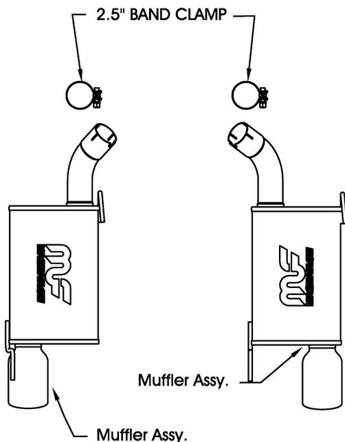
**Step 2:** Remove the OEM hanger brackets from the mufflers and reattach them to the frame of the vehicle. Install the new mufflers by fitting the welded hangers into the rubber insulators in the brackets. Fit the new mufflers to the overaxle pipes using the supplied band clamps. Leave all the clamps and fasteners loose for the final adjustment of the complete system.
