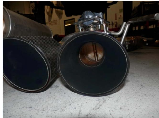
**Step 4.** Before installing your new exhaust system attach the OEM valve motors to each valve using the supplied M5 hardware. The alignment spring on the motor will need to be engaged into the keyway slot of the new valves.
