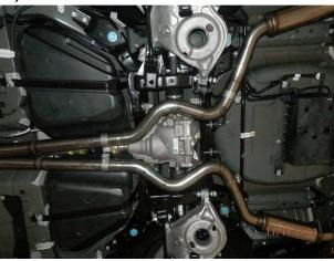
**Step 3.** Next attach the Extension Pipe Assemblies to the Y-Pipe using the supplied 2.50" clamps and fitting the hangers into the rubber insualtors.
