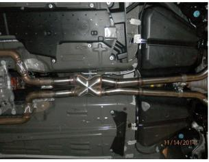
**Step 2.** Begin installation of the new system by loosely attaching the X-Pipe Assembly to the outlets using the OEM clamps. Leave all clamps loose until final adjustment.
