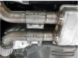
**Step 1.** (Notice: This exhaust system fits on both convertible and coupe Mustangs. To install the system on a convertible you must first remove all underbody bracing.) Begin removing the exhaust system by loosening the clamps located in front of the resonator. Next, working front to rear extract the hangers from the rubber insulators and remove the OEM system. Retain insulators and clamps as they will be used to install the new system.
