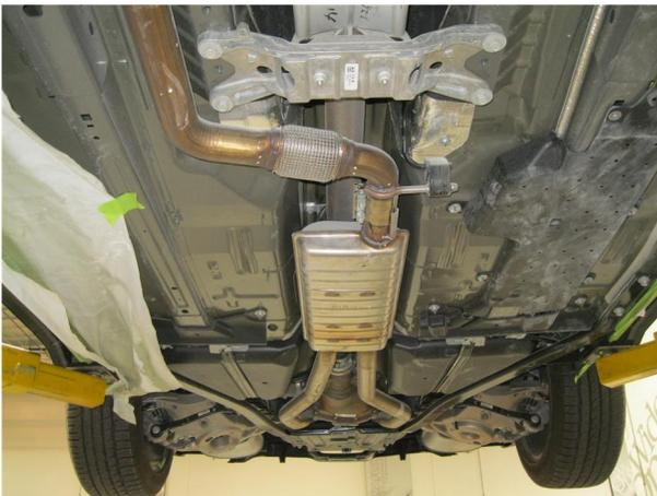
**Step 1.** (Notice: This exhaust system fits on both convertible and coupe Mustangs. To install the system on a convertible you must first remove all underbody bracing.) Begin removing the exhaust system by loosening the clamp located in front of the resonator. Next, working front to rear extract the hangers from the rubber insulators and remove the OEM system. Retain insulators and clamps as they will be used to install the new system.
