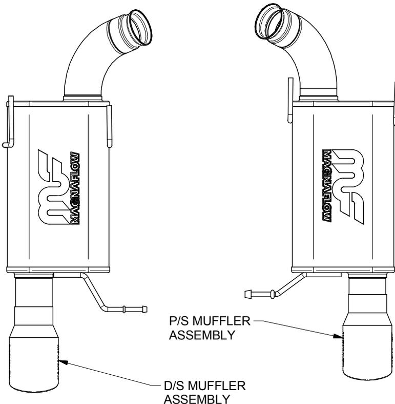
**Step 1:** (Carefully read all instructions before installation) To remove the OEM mufflers, first locate the ball flare clamp assembly attached to the inlet section of both mufflers. Remove the clamp from both the passenger and driver side, then remove the hangers from the rubber insulators. (three on each side). (Do not damage the OEM rubber insulators or clamps as they will be reused to mount your new Magnaflow system)
