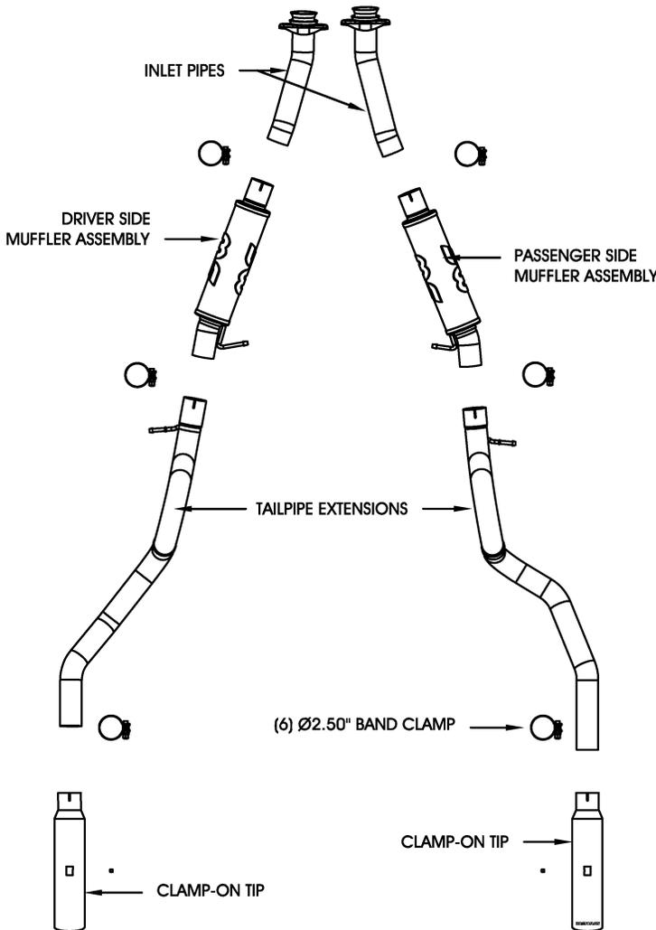
**Step 1:** To begin removal of your OEM exhaust system, you will need to cut the tail-pipes just behind the mufflers. Remove the tail pipes from the OEM rubber insulators. Do not damage the rubber insulators, as they will be re-used with your new system. Next unbolt the extension pipes from the H-pipe and remove the mufflers from their OEM rubber insulators. Do not discard the fasteners required to bolt the extension pipes to the mufflers, as they will be re-used.
