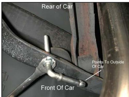
**Step 6:** With all components mounted loosely, adjust the system for overall aesthetics and clearance of frame & bodywork. (MAGNAFLOW recommends at least 1/2" of clearance between the exhaust system and any body panels to prevent heat-related body damage or fire.)
