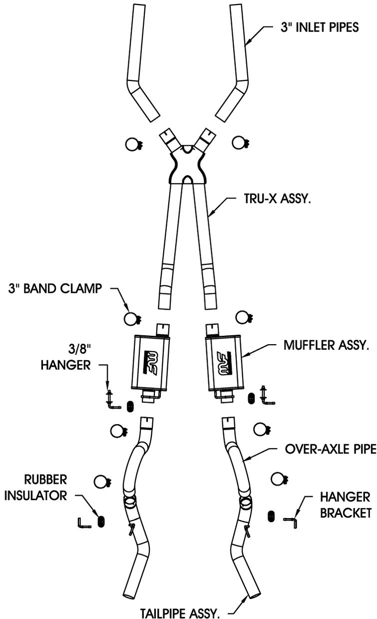
**Step 1:** (Carefully read all instructions before installation) Disconnect the battery before removal of the existing exhaust system. Remove the existing exhaust system from the exhaust manifolds / headers. Some systems may need to be cut for removal. Take notice of axle position and brake line position.
