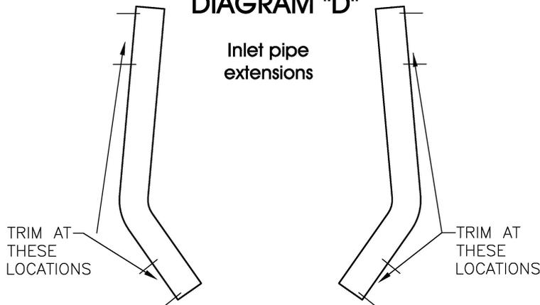
*Note: This system is designed to work with OEM-style exhaust manifolds, or tubular headers. Due to the various applications possible, some modification and welding is required for a proper fit and finish.*
