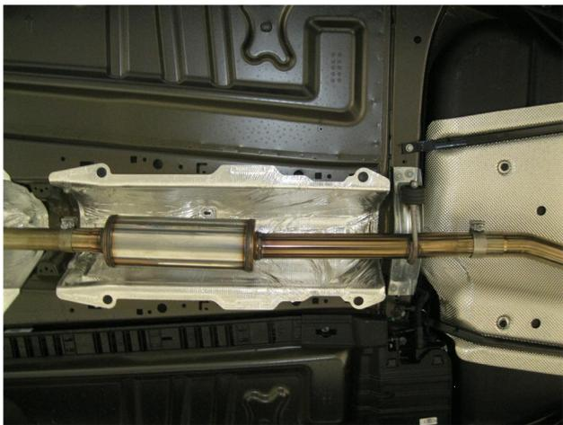
**Step 2.** Begin installation of the new system by fastening the Resonator Assembly inlet to the catalytic converter using the supplied 2.25" clamp (Leave all clamps and fasteners loose for final adjustment of the complete system).
