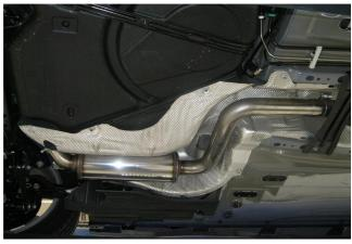
**Step 4.** Slip the inlet of the Muffler Assembly over the outlet of the Inlet Resonator Assembly and loosely secure using the supplied 2.50" band clamp. The supplied rubber insulated will be needed on 2015 applications only. Install the Tail Pipe Assembly in a similar fashion.
