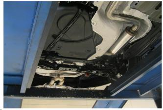
**Step 5.** With the complete system loosely mounted to the vehicle locate the supplied Hanger Bracket to the rubber insulator. Next, bolt the hanger Bracket to the Tip Y-Pipe Assemble using the supplied hardware.
