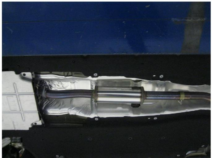
**Step 3.** Begin installing your new system by loosely attaching the inlet flange of the Resonator Assembly to the catalytic converter outlet using the OEM fasteners.
