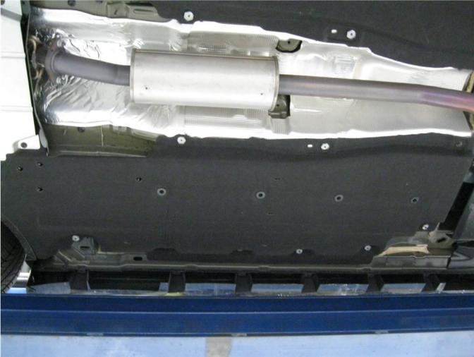
**Step 1.** Begin removing the OEM exhaust system by unbolting the flange at the catalytic converter outlet. Retain the mounting hardware as it will be needed to install your new system.
