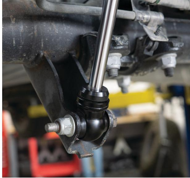
Fig. 16: Install the lower shock bolt.
