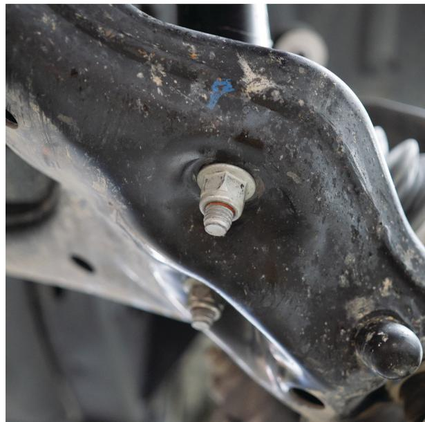
Fig. 7: Remove the bar-pin bolts.
