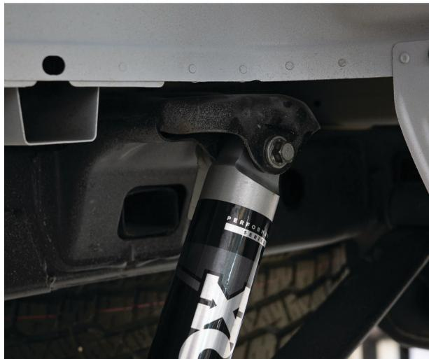
Fig. 15: Install the upper shock mount.
