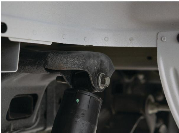
Fig. 13: Remove upper shock mount bolt.
