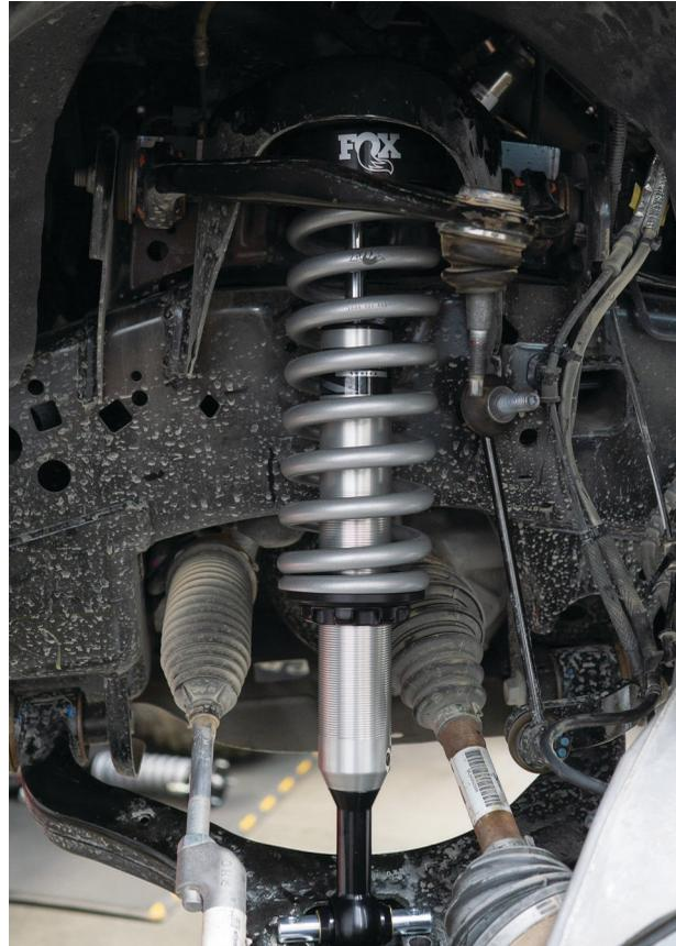
Fig. 8: Install FOX coil-over.
