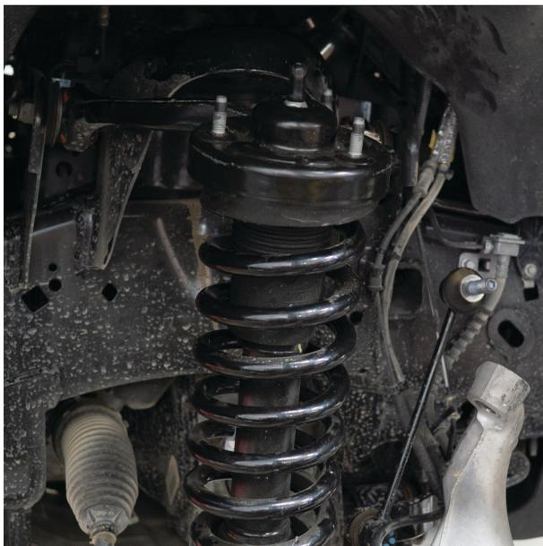
Fig. 6: Free the coil-over.
