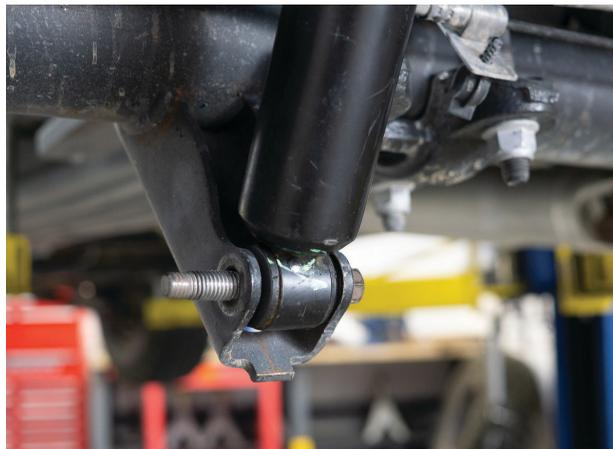
Fig. 14: Remove lower shock mount bolt.
