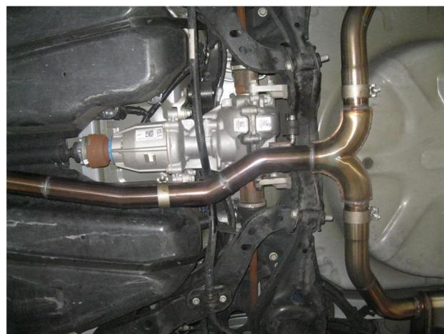
**Step 3.** Next attach the Mid-Pipe Assembly to the Resonator, followed by the Y-Pipe Assembly. Use supplied 2.50" clamps and fit hangers into rubber insulators.
