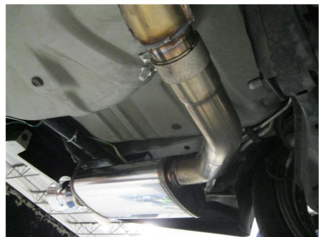
**Step 4.** Finish by installing both Muffler Assemblies using the supplied 2.50" clamps, fitting the hangers into the rubber insulators.
