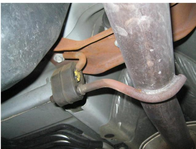
**Step 1.** begin removal of the OEM system by loosening the clamp at the outlet the flex pipe. Working front to rear detach all hangers from rubber insulators and remove the system. Retain rubber insulators as they will be re-used the mount the new system.
