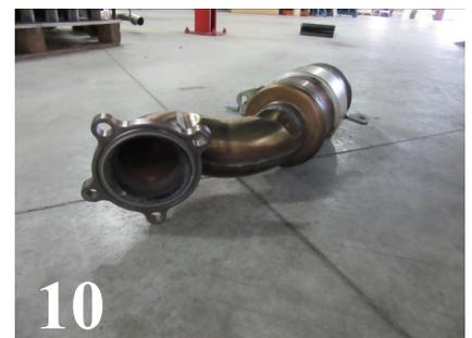
**WARNING:** *Use extreme caution during installation. Torque all fasteners according to manufacturer's torque values and tightening sequence. **DO NOT** use air impact tools to tighten fasteners on Borla Performance Exhaust Systems. Use of such tools may result in bent flanges or gasket contact areas leading to exhaust leaks.*
