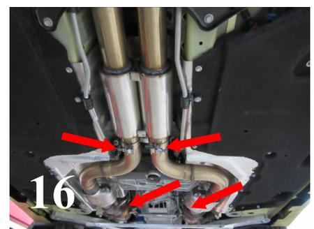
**WARNING:** Use extreme caution during installation. Torque all fasteners according to manufacturer's torque values and tightening sequence. **DO NOT** use air impact tools to tighten fasteners on Borla Performance Exhaust Systems. Use of such tools may result in bent flanges or gasket contact areas leading to exhaust leaks.
