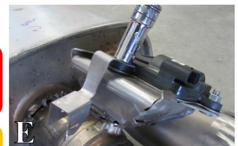
**WARNING:** Use extreme caution during installation. Torque all fasteners according to manufacturer's torque values and tightening sequence. **DO NOT** use air impact tools to tighten fasteners on Borla Performance exhaust systems. Use of such tools may result in bent flanges or gasket contact areas leading to exhaust leaks.
