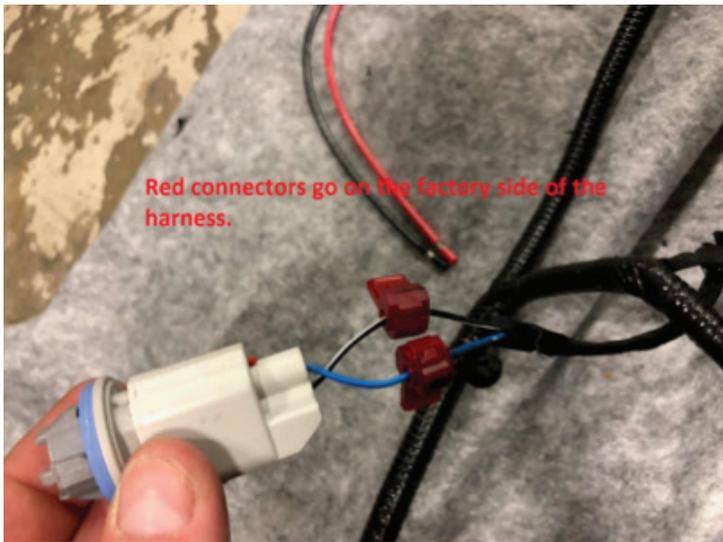
2. \*When experiencing a hyper flash or when replacing halogen lights with led lights a resistor should be used. The resistor will wire into the positive power supply to the light and the negative side of the ground supply to the light.
