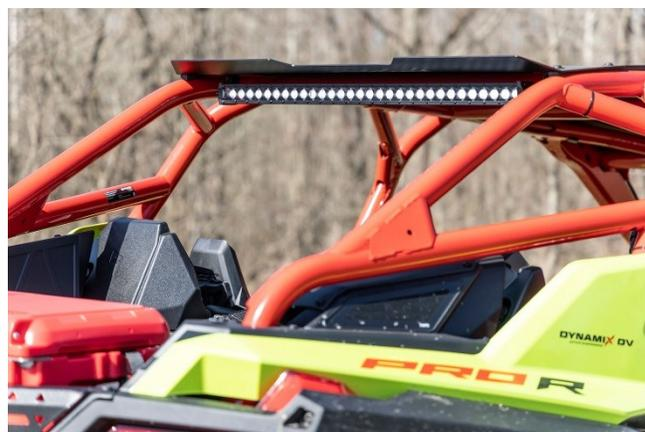
5. Install the light bar to the brackets using the hardware supplied with the light. **See Photo 5.**
