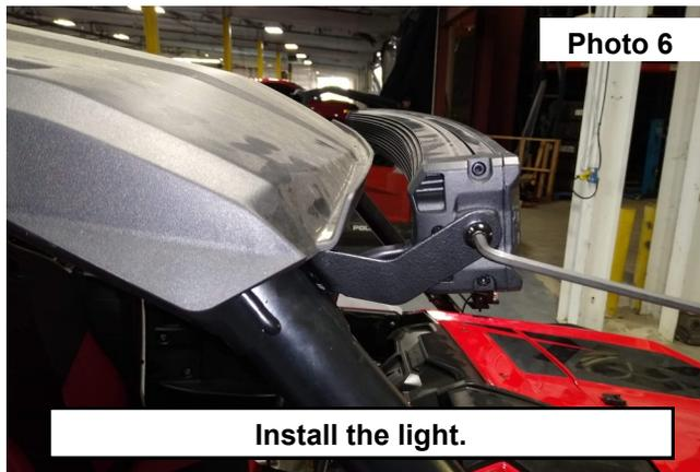
8. Tighten the Driver and Passenger light bar bracket to the cage using a 13mm wrench and socket.
