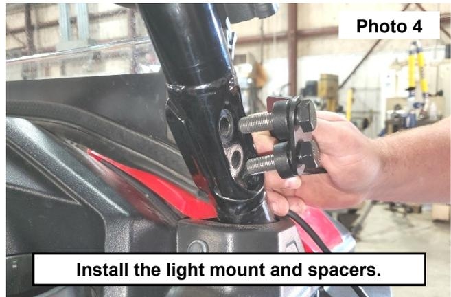
6. Repeat the installation of the light and mount on the opposite side.
