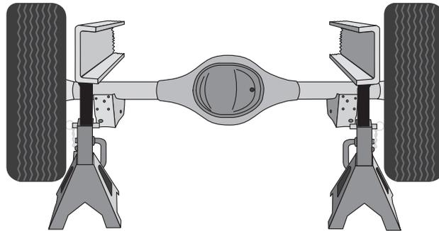
2. Some models may have a rubber isolator at the top of the passenger's side coil spring. This isolator needs to be removed and can be discarded (Fig. 2).
