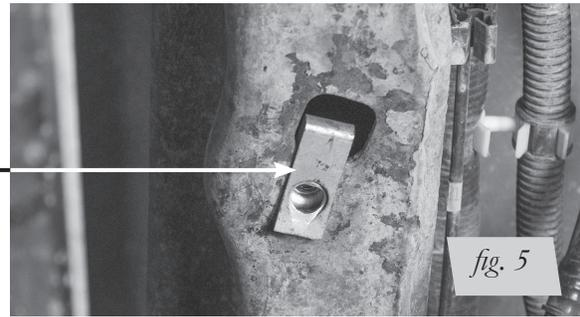
5. All years: On the right side (passenger side) there is an emergency brake cable holder that is bolted on to a bracket welded to the axle, with a self-tapping bolt. In order to make clearance for the axle strap, it will be necessary to cut this off and/or grind this bolt flush to the bracket (Fig. 6).
