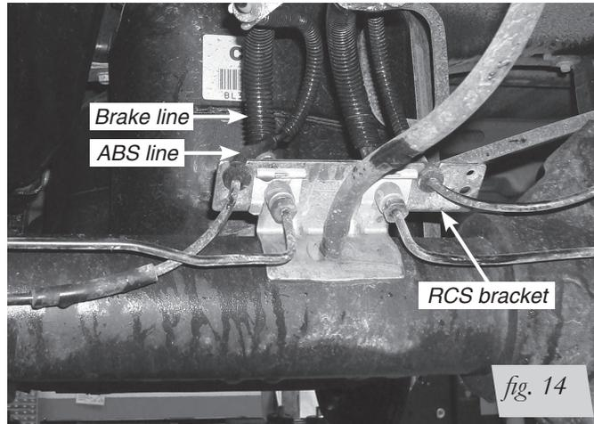
2. Remove the right ABS line out of the bracket by pulling it straight up (Fig. 15).
