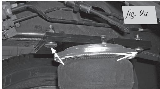
*Left hand assembly (driver side) attached with carriage bolts (R), flat washers (M) and nylon lock nuts (U). Torque to 31lb.-ft.*
