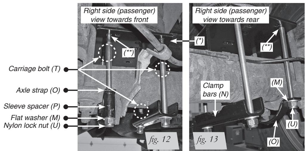
(\*) Push the bracket against the leaf spring in between the stock U-bolts.
