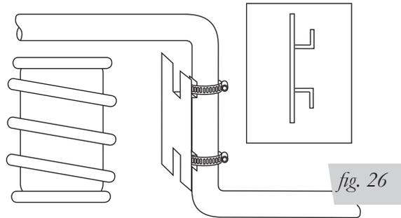
4. Bend the heat shield to form it around the tail pipe. Be sure to maintain a "dead air" space of 1/2" to 1" between the tail pipe and the heat shield (Fig. 27).
