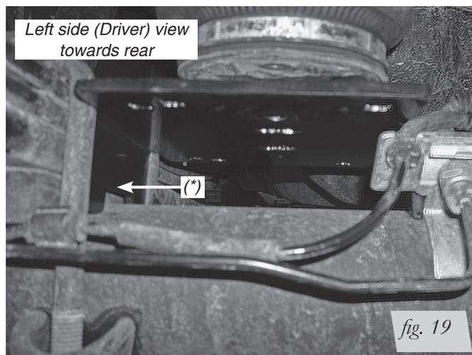
(\* Push the bracket against the leaf spring in between the stock U-bolts.
