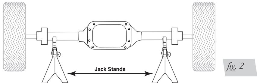
2. Drop the axle or raise the frame up to make room for the assemblies to be put into position between the frame and axle.
