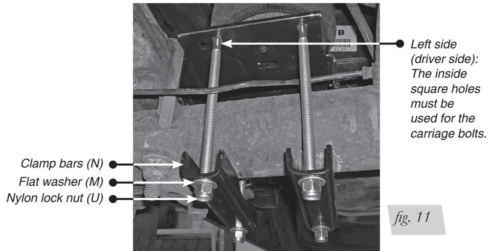
3. Install the lower clamp bars (N) over the carriage bolts installed previously and cap with flat washers (M) and nylon lock nuts (U) (Fig. 11). Torque the lower nuts evenly to 10 lb.-ft.
