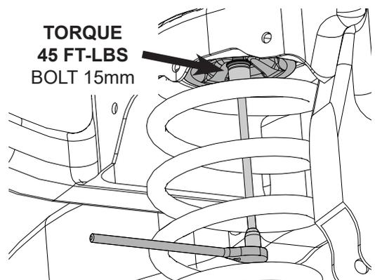
TIP: USE AN EXTENSION TO HELP TIGHTENING / TORQUE BOLT
