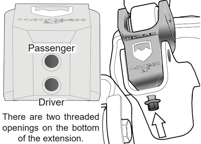
There are two threaded openings on the bottom of the extension.
