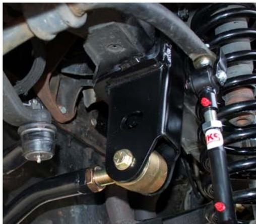
5. Front install should be complete, however keep everything loose at this time until rear is lifted, then final adjustments can be made and everything can be tightened.
