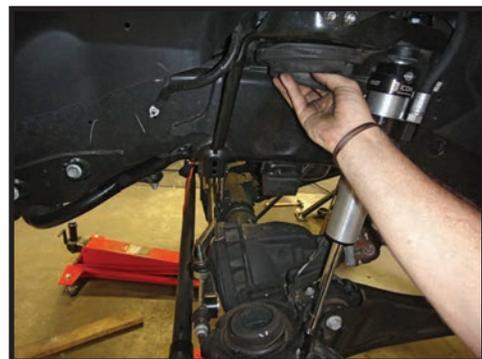
**5.** Slowly lower the axle with the support jack until both driver and passenger springs become free. Remove the factory coil springs, leave the factory rubber isolators installed and located with the locating nipple in the upper coil bucket. **(FIGURE 4)**
