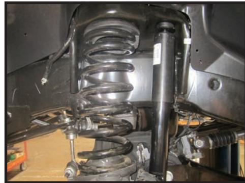
4. Remove the sway bar links from the sway bar using a 10mm and an 18mm. (FIGURE 3)
