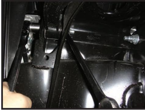
**8.** Before installing your new upper control arms, care must be taken to grease the bushings (liberally) prior to installing assembly. Failure to grease properly will cause premature bushing wear and increased noise. [FIGURE 3]
