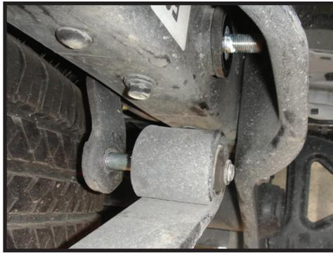
**9.** Remove the shackle from the inside of the frame rail. This may require removal of the spare tire.
