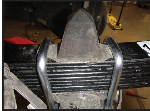
**14.** Install the U-bolts and tighten. [FIGURE 4]
