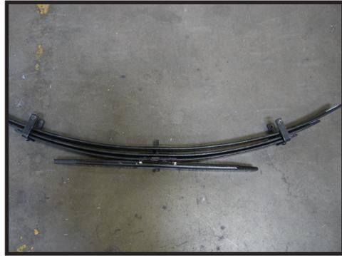
**9.** Tighten one side of the C-Clamps and threaded locating pins slightly, then the other side, back and forth till the springs are fully clamped together.
