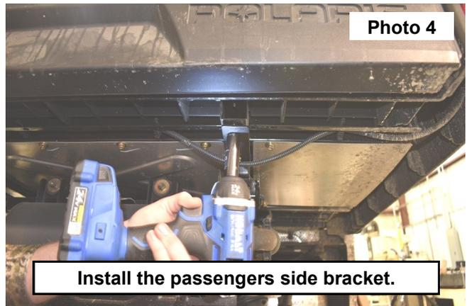
5. Install the passengers side bracket with the mounting tab to the inside of the UTV. Secure using (2) of the supplied 5/16-18 self tapping bolts. Tighten using a 13mm socket. **See Photo 5.**
