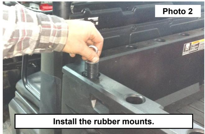
3. Install the top of the rubber mount just below the taper in the top of the bed. Then remove the eye bolt and washer. Retain for reuse. **See Photo 3.**
