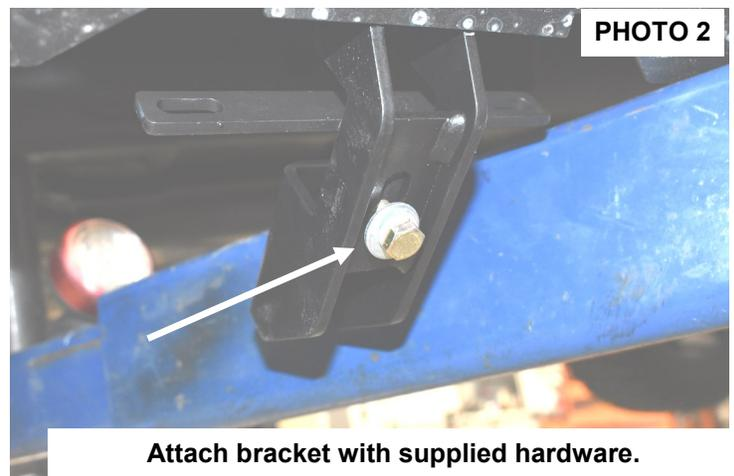
Attach bracket with supplied hardware.
