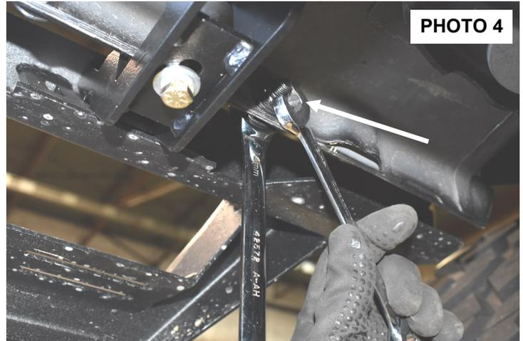
7. Tighten the 8MM x 35mm bolts and then tighten the 8mm x 25mm bolts using a 13mm wrench.
