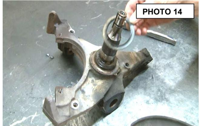
18. Place dust shield on new spindle using stock hardware. Tighten with 13mm socket. **See Photos 16 & 17.**
