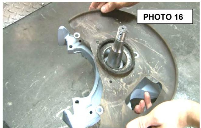
19. Place new drop spindle on lower ball joint. Place factory nut on lower ball joint and hand tighten.
