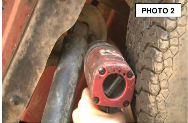
1. Using 18mm socket and wrench, remove lower shock bolt. **See Photo 1.**
