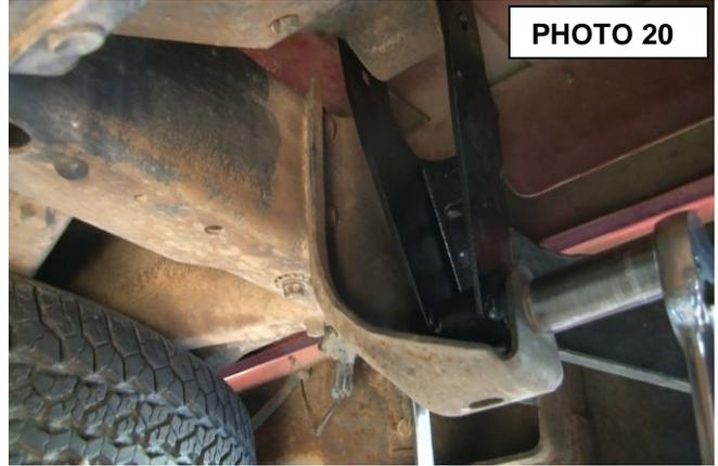
20. Using 13mm socket and wrench, install factory upper hardware in Rough Country N2.0 shock. Tighten to factory spec. **See Photo 21.**
