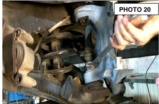
21. Using a 21mm wrench, tighten upper ball joint. **See Photo 19.**
