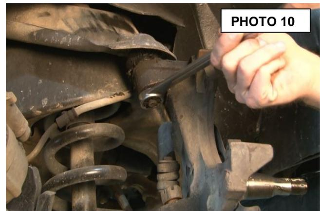
13. Strike front side of knuckle at upper ball joint to loosen. Once the upper control arm pops up, remove nut from ball joint. **See Photo 11.**
