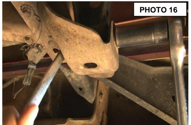
16. Using 22mm socket and wrench, remove upper shackle bolt. **See Photo 17.**
