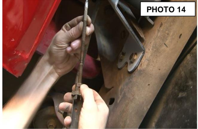
15. Using 22mm socket and wrench, remove lower shackle bolt. **See Photo 16.**
