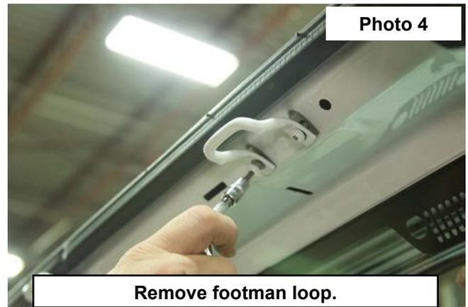
7. Install the switch pod bracket and footman loop using the stock hardware and a T25. **07-08 models will install the bracket that was not attached to the switch panel, using the supplied rivets. See Photo 5.**
