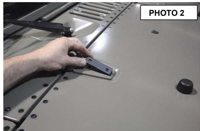
3. Install hood bracket on top of the spacer and secure with the 8mm bolts as shown in **Photo 3**. Repeat on driver side.
