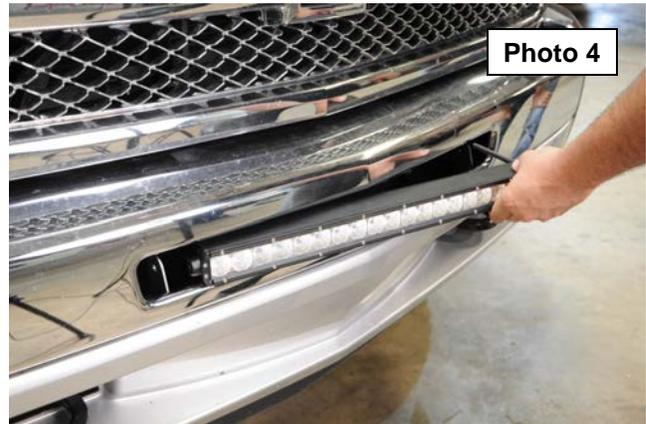
5. Make sure light and bracket are centered in bumper and tighten the 3 bolts holding the bracket in.
