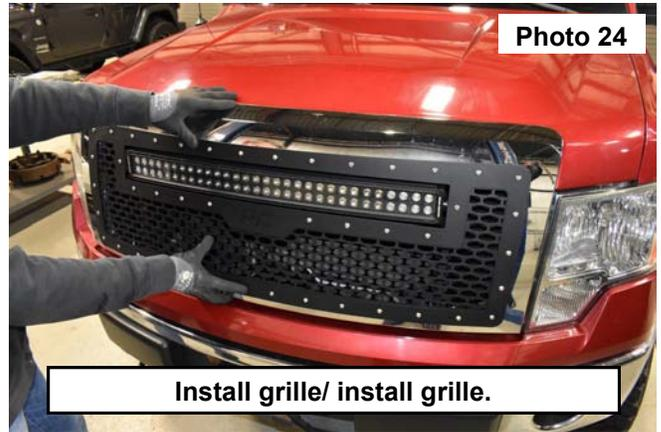
29. Install the removed nuts at the top of the hood securing the grille into place, tighten using a 10mm socket. **See Photo to 25.**
