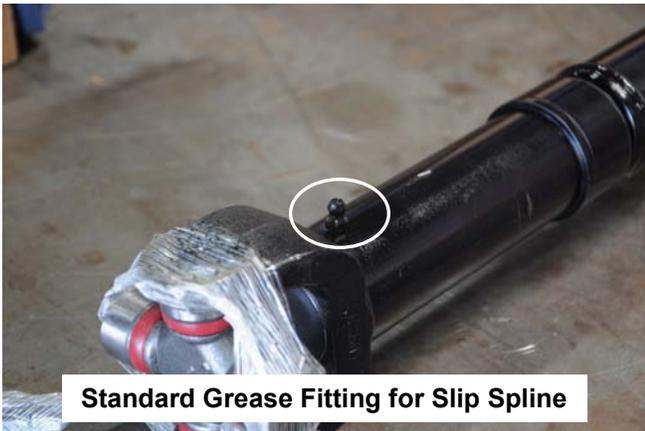
**Standard Grease Fitting for Slip Spline**
