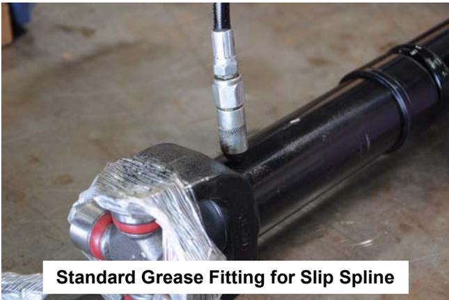
**Standard Grease Fitting for Slip Spline**
