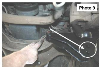
19. Using a 32mm socket, attach the upper end of the track bar to the new bracket in the upper hole for the 4" lift, lower mounting hole for the 6" lift—see PHOTO 9. Using the factory hardware. Insert the bolt from the front to the rear and hand tighten only, it will be tightened in a later step.
