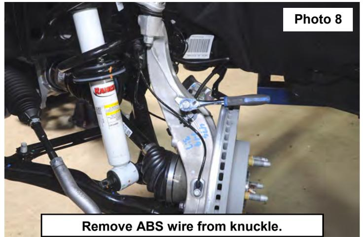
13. Using a 10mm socket, remove the ABS sensor from the knuckle. Retain hardware and hang ABS wire out of the way. **See Photo 9.**
