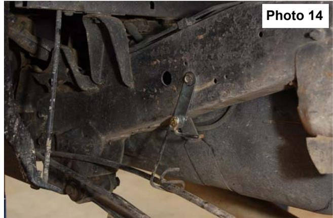
9. Install wheels and lower vehicle on the ground and tighten leaf spring bolts using 21mm socket and wrench. Tighten lower control arm bolts using 21mm socket and wrench.
