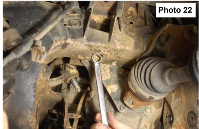
25. Remove both bumper stops from frame using 13mm socket
