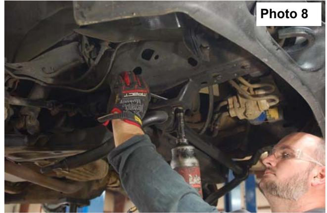
7. Remove the abs and brake line from upper control arm using two 13mm wrenches
