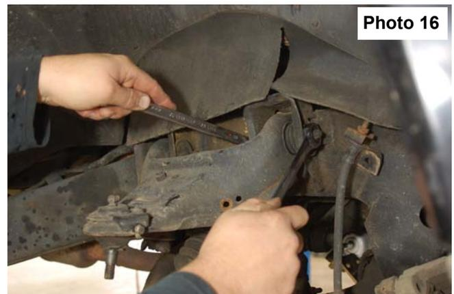
18. Removing the lower control arm using a 21 mm socket and wrench. **See Photo 17.**
