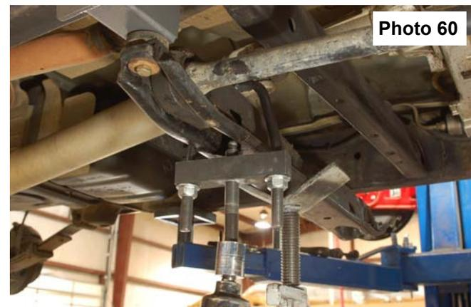
55. Install transfer case skid plate if equipped with stock hardware.
