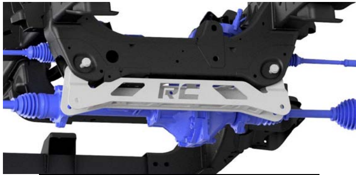
Install front crossmember.
